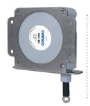
The SG1 uses a precision high-cycle plastic hybrid potentiometer and an extremely durable spring-loaded stainless steel measuring cable to provide an accurate reliable position feedback signal over the entire stroke.
