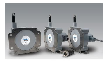
The SG1 provides absolute linear position up to a 10-ft. stroke range. Constructed with a rugged polycarbonate body, this model is available in an 80-inch or 120-inch stroke range and offers optional IP67 protection for wet or outdoor installations and an M12 connector for easy installation.
